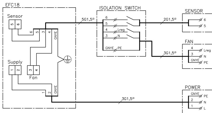
Connect the EFC18 and the temperature sensor as in the diagram below (RSHT).
