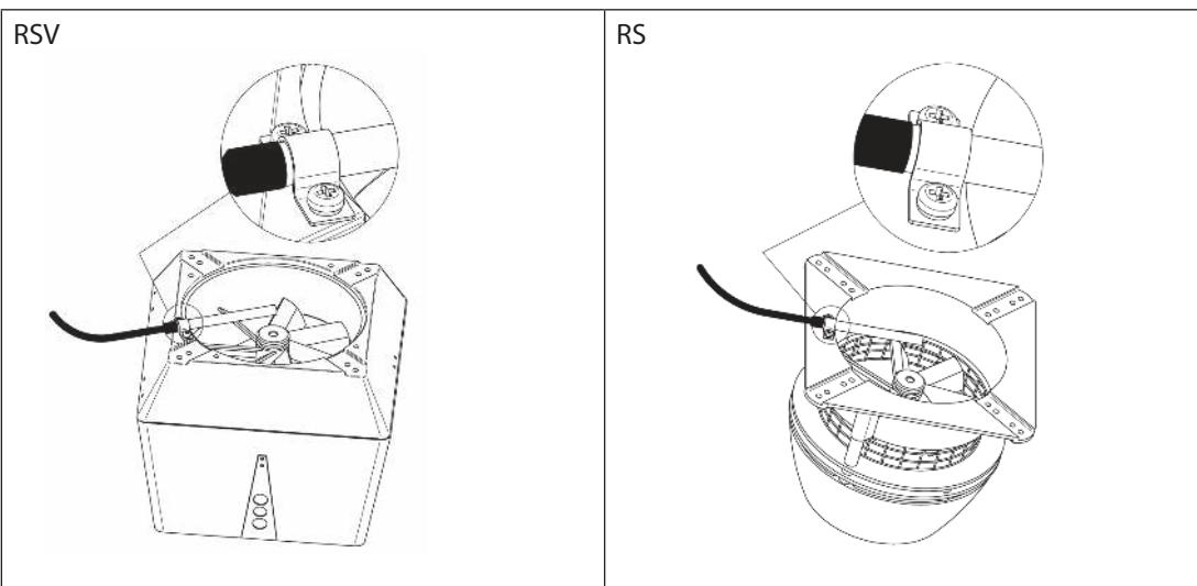
If an FRx-AFD flange is used: Remove the plug from the pipe, and insert the sensor. Tighten the screw (A).
