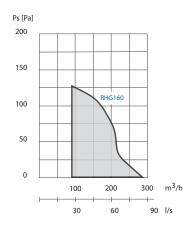
The capacity diagram is measured at a flue gas temperature of 20 °C. The fan capacity changes with temperature.
